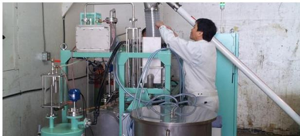
**Investing in innovation:** A machine that converts plastic into crude oil is up and running in Whitehorse. The first of its kind in North America, the machine at P&M Recycling is already producing enough oil to heat the recycling centre it is housed in.
